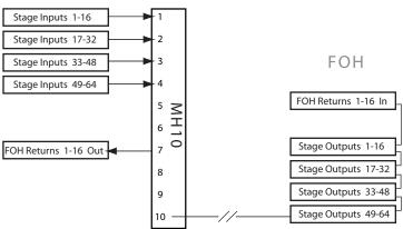
A 64x16 digital snake using only one MH10 Merger Hub
